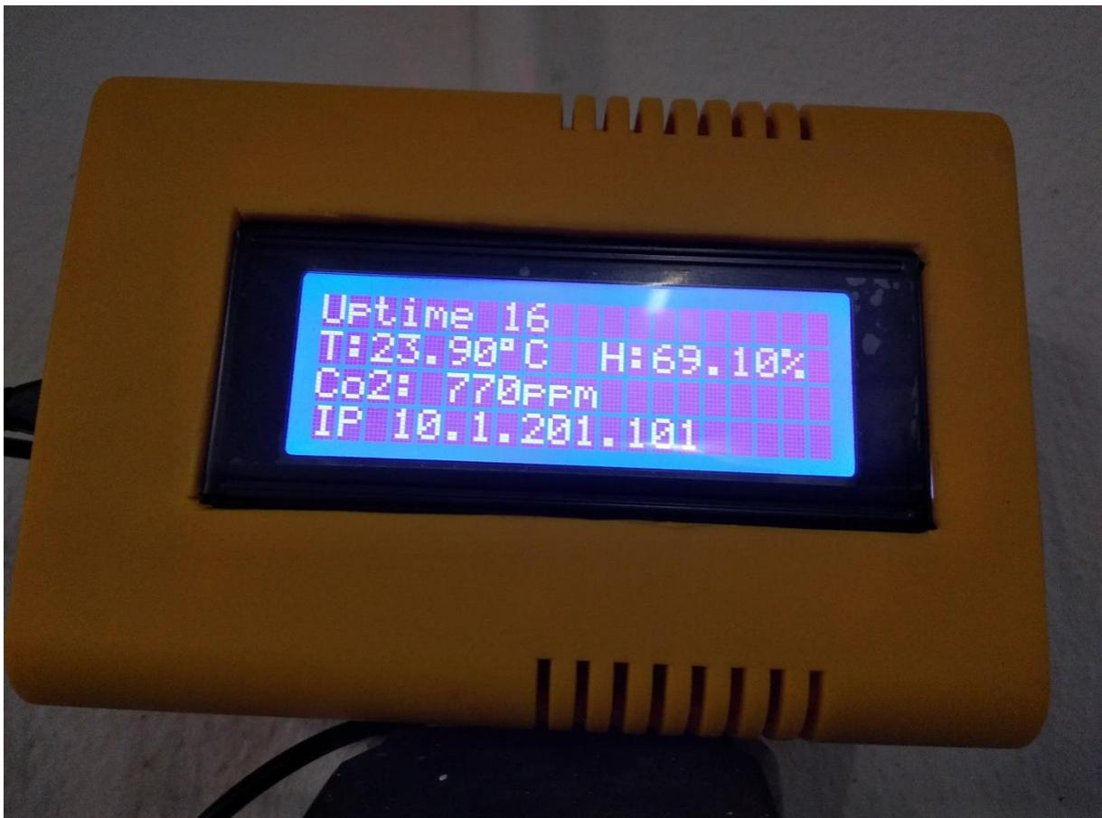
The rigged setup now runs over 1,5 years under roughest conditions and still works perfect, which really is remarkable for a gas sensor thanks to the robust design of the S8.
